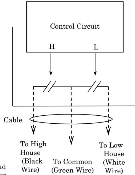
The Autopuller connects the wires together using a control circuit. Pressing the High button connects the high wire to the common wire. The same process for the Low and Both. This is the same as the existing pull head.
