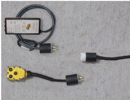
The photo above shows how the original pull cord was modified using twist lock connectors. This allows either the original head or a wired Autopuller to be used with the same cord.
