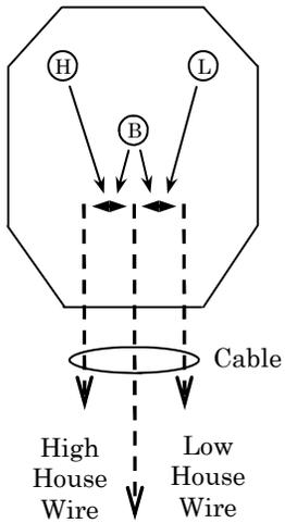
Pressing the High button will connect the high wire to the common wire. (Same for low) The Both button will connect all three wires together.
