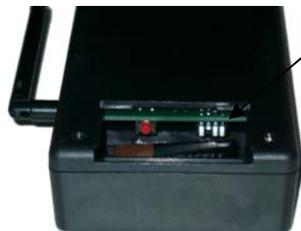
As seen thru opening, Right 2 switches set machine signal
