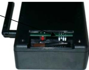
As seen through opening, right 2 switches set machine signal
