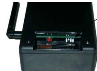
As seen thru opening, Right 2 switches set machine signal
