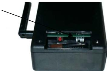
As seen thru opening, Right 2 switches set machine signal
