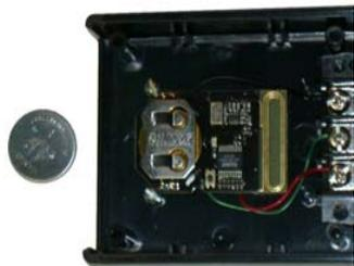
Step 3 Slide the battery out of the its holder.
