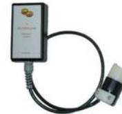
Step 3 Install the mating connector on the wire. You may have to open the connector on the Autopuller to identify which wire is on which terminal.
