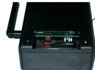
As seen through opening, right 2 switches set machine signal
